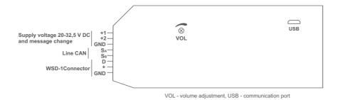
Providing the supplay voltage to: input +1 will play message K1.mp3, input +2 will play message K2.mp3, inputs +1 and +2 at the same time will play message K3.mp3
